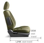
This information is so you can establish the forward and back movements of the seat with the LINK. In all applications, the LINK adds power forward and backward movements, regardless of the seat's original functions. In some applications, the travel is limited. The seat adjustment information will allow you to confirm if the installation of the LINK will be suitable for your client's needs.
